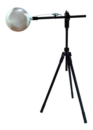
Caution: in order to avoid the overturning of the tripod given to the weight of the test head, make sure that the two first extension elements of the legs are open and that the T junction mod. P-0007 is mounted as in the picture.
