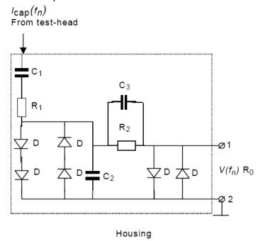
Where: C1=470 pF; C2=10 nF; C3= chosen in calibration; R1=470  $\Omega$ ; R2=150  $\Omega$ ; D=diodi schottky.
