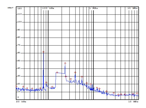
The MSA-210 equipment is used for the measurement of the current density induced by the electromagnetic field emitted by the device that is being tested. Follow the verification method specified in IEC 62493 D and E appendices; The device under test complies with IEC 62493 if F≤0,85 where F is represented by the formula E.4
